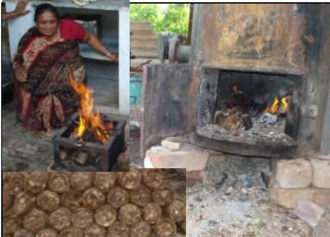
Briquettes (3900 kcal/kg) being used to fire the boiler. The steam is used for oil expelling and other applications. The ash is ploughed back into the field. The briquettes also burn nicely in a chuhla with low smoke.
