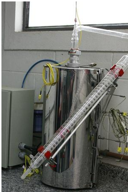
Reformer (Ethanol) for hydrogen production
