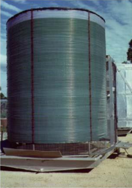
A 1000 L helical tubular photobioreactor at Murdoch University, Australia. Courtesy of Professor Michael Borowitzka, Murdoch University
