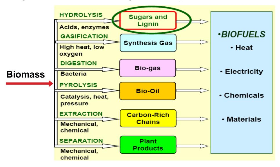
Fermentation of residues and waste to Biogas
