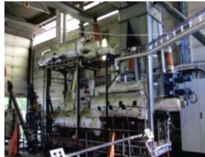
Rotary drum / Auger (Umeå University) pilot
