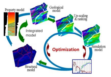
Field optimization framework – coupling of reservoir and facility models
